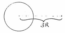
Find the difference in the electric potential between a point a distance 3R from the center of the sphere and a point at the center. Which point has the higher value of the electric potential?
