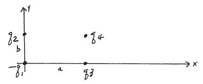
The distances a and b are known. The charge at the origin is known and negative,  $-q_1$ . The charge  $q_2$  at x=0,y=b is unknown. The charge  $q_3$  at x=a,y=0 is unknown. What must be the unknown charges  $q_2$  and  $q_3$  if the electric force on a positive charge  $q_4$  at x=a,y=b is to be zero?
