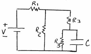
Solve for the charge on the capacitor for the special case where  $R_1=0.$
