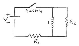
a. If the switch has been closed for a long time so that the steady state has been reached, find the currents in the resistors.
