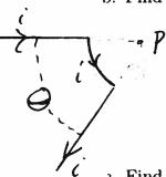
c. Find the magnetic field at the point marked P which is at the center of the circular segment that has radius W.
