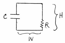
a. Derive the equation, starting with a law, that could be solved for the charge on the top plate of the capacitor. No credit will be given if the direction of the current and the charges on the capacitor plates are not indicated on the figure.
