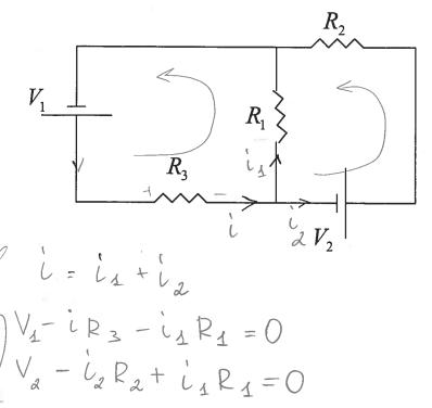
b) Find the current through resistor  $R_2$  assuming that  $R_1 = R_2 = R_3 = R$  and  $V_1$  and  $V_2$  are given.
