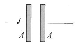
The electric field is a function of time  $E = E_0 \cos \omega t$ . Find the current i in the wire and show that it is equal to the displacement current between the plates.
