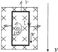
a) Find the current in the loop as a function of the velocity v if the loop is falling down but is completely within the region having magnetic field  $\vec{B}$ .
