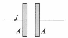
The electric field between the plates is a function of time  $E = E_0 \cos \omega t$ . Find the current i in the wire and show that it is equal to the displacement current between the plates.
