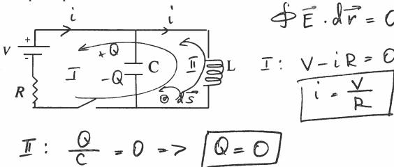
b) At t=0 the switch is opened. Find the charge on the capacitor as a function of time. (Assume that L includes self-inductance).
