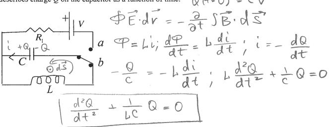
b) Solve for the charge on the capacitor as a function of time.
