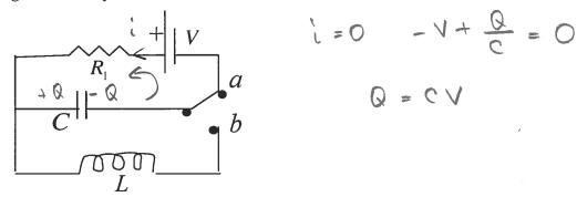
b) The switch is then thrown to position b. Starting from some famous law, derive the equation that describes charge Q on the capacitor as a function of time. 12(4=0) = CV
