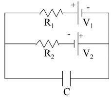
Find all currents, voltage drops across the resistors, and the charge on the capacitor plates.
