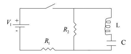
a) If at *t*=0 the switch is opened, what differential equation **can be solved** to find Q, the charge on the capacitor, as a function of time? (Assume that L includes the self-inductance). **Do not solve the equation.**
