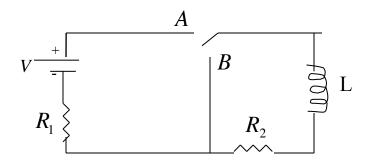
d) At t=0 the switch is moved to the position B. Find the current through  $R_2$ , as a function of time. (Assume that L includes self-inductance).
