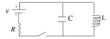
b) At t=0 the switch is opened. Find the charge on the capacitor as a function of time. (Assume that L includes self-inductance).
