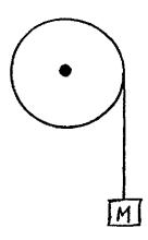
b. Suppose there is a friction force at the axle which exerts a torque, opposing the rotation and that this torque is proportional to the angular velocity, with magnitude  $\beta\omega$  where  $\beta$  is a known constant. The pulley will then reach a certain constant angular velocity. What is this constant value of  $\omega$ ?
