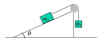
c) Assume that the surface of the inclined plane of a given angle  $\theta$  is frictionless, but the pulley has radius R and moment of inertia *I* with respect to the axis of rotation. The string pulls without slipping. In the box below write the system of equations that can be solved to find the acceleration of the block  $m_1$ .
