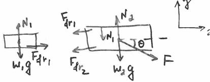
b) What is the maximum magnitude  $F_{\text{max}}$  of the force at which the two blocks still move together with the same acceleration?
